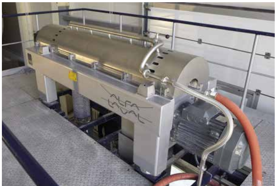
Dewatering kieselguhr using a Foodec decanter centrifuge
