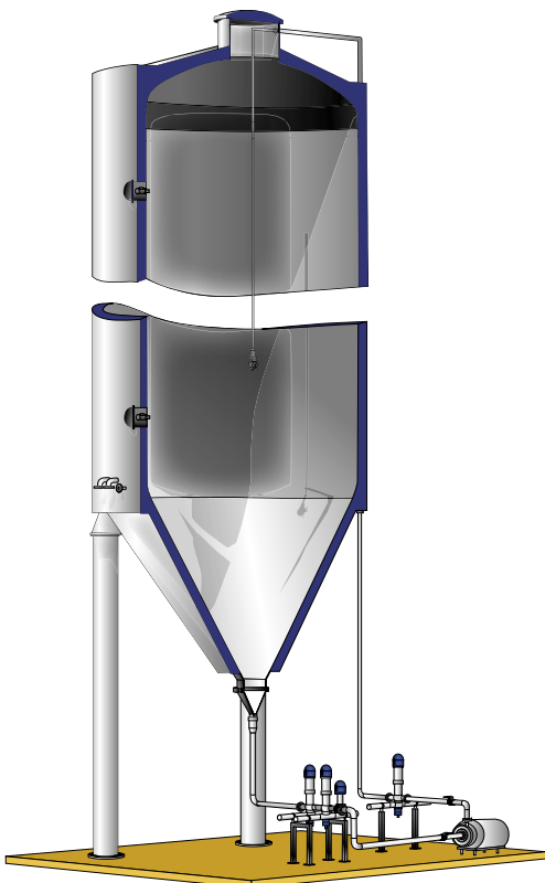
Illustration of Iso-Mix fermentation system
