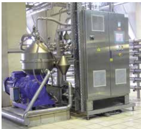
Beer recovery using a BRUX 510 nozzle separator
