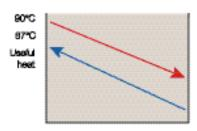
Thanks to its crossing temperatures and very close temperature approach, a compact heat exchanger is able to recover virually all of the incoming heat (above). With a shell-and-tube, this is not possible – by design (below).
