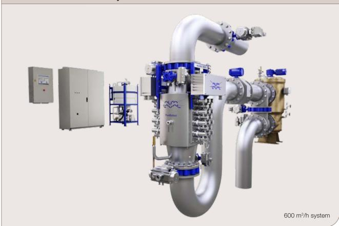
Alfa Laval PureBallast 3.1 is an automated inline treatment system for the biological disinfection of ballast water. Operating without chemicals, it combines initial filtration with an enhanced form of UV treatment to remove organisms in accordance with stipulated limits.
