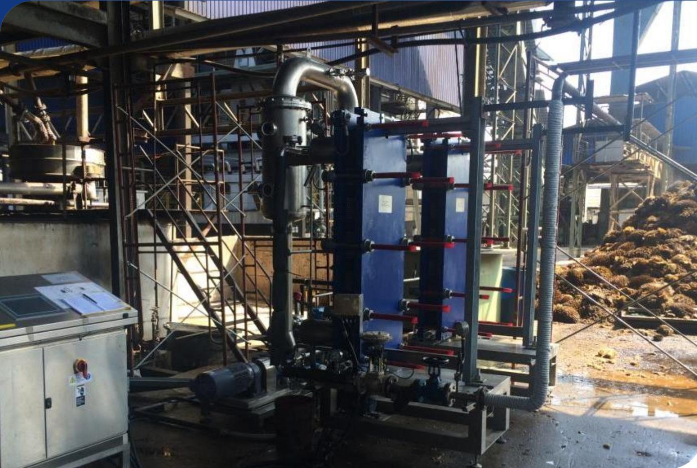
To develop the POMEVap solution, Alfa Laval has tested the POME concentration using Alfa Laval's evaporation test unit for an extended trial period ( $\approx$  4 weeks) at customer mill sites in Malaysia
