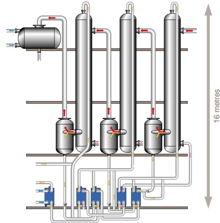
Shell-and-tube falling film evaporator
