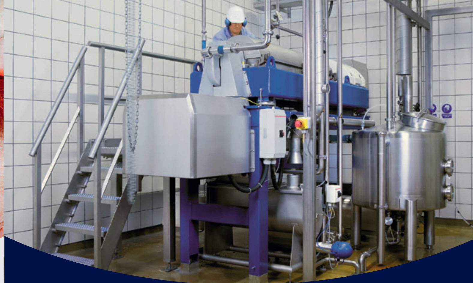
Decanter centrifuge system for protein processing
