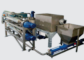
CentriFlow - wet rendering module
