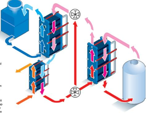
Heat recovery is a good example of the kind of system optimization in which Alfa Laval has years of experience. In an optimized HVAC system waste heat from cooling can be used to warm for example tap water. With Alfa Laval plate heat exchangers it is possible to recover up to 95 percent of energy that would otherwise be wasted.
