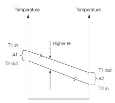
The diagram shows that small temperature differences result in high theta.
