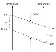
The diagram shows that large temperature differences result in low theta.
