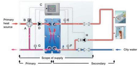
valve accordingly, via the control box, in order to supply domestic hot water at the right temperature.
